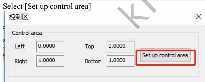
Adjust the screen area controlled by this radar (blue is the control area) by adjusting the four values of left, up, right and down.
