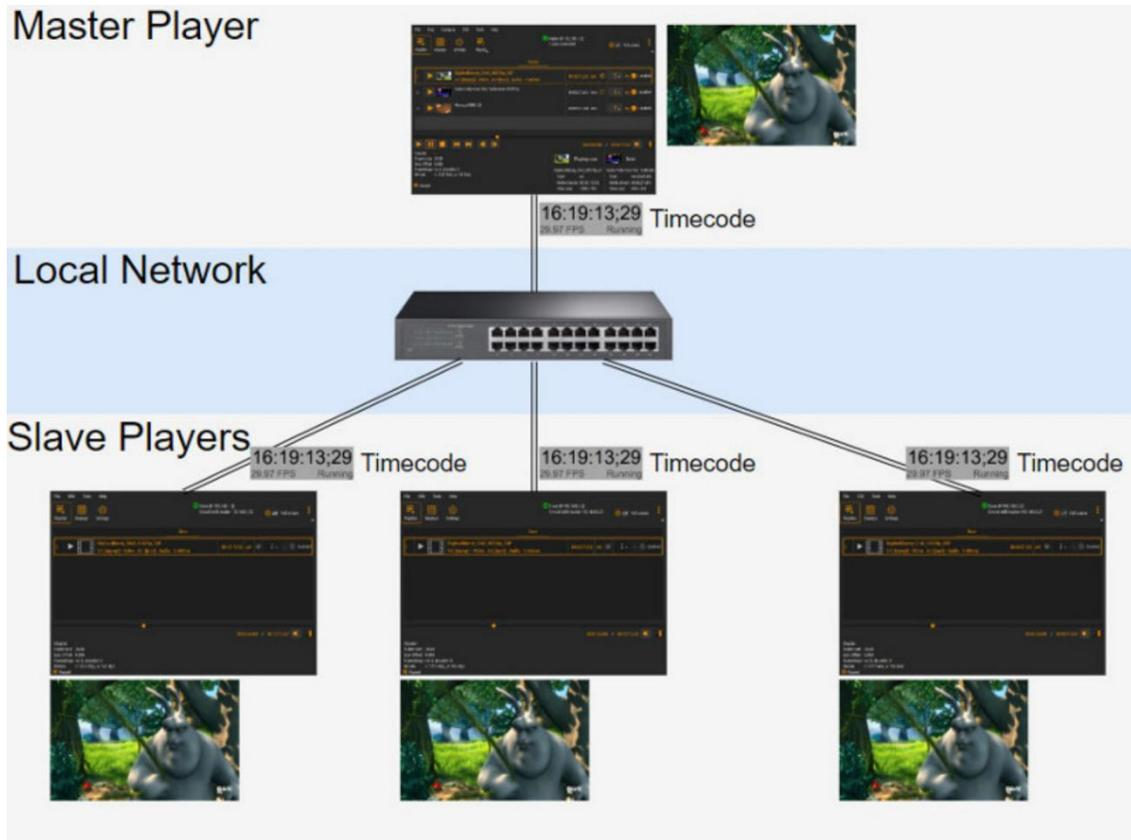
This synchronized distributed playback can be used in huge video wall setups like this one. The large video media can be split in multiple sections and each smaller section can be played back on one PC connected to one or more displays.
